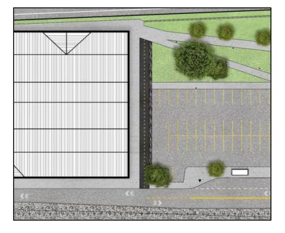
Segment 2 includes one of the constricted segments for the trail along North Marginal Road, as the existing path narrows to 11 feet between North Marginal Road and the Burke Airport fence on the curve north of the Muni Lots Road interchange. Along trail segments with constrained right-of-way, the trail will typically need to be situated immediately next to North Marginal Road. A 2 foot brick paver can be used to demarcate an 8 foot path from North Marginal Road, and add aesthetic interest.
