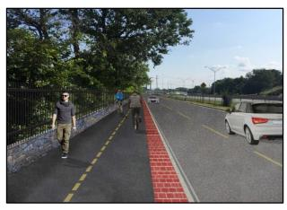
Top right: a stone wall and fencing treatment is proposed along the Yacht Club frontage. At a width of 8 feet, the path is less than the width of 10 feet recommended by AASHTO; a slight shift in roadway alignment could create the space needed for greater width, if desired. Below: trail along South Marginal Road.
