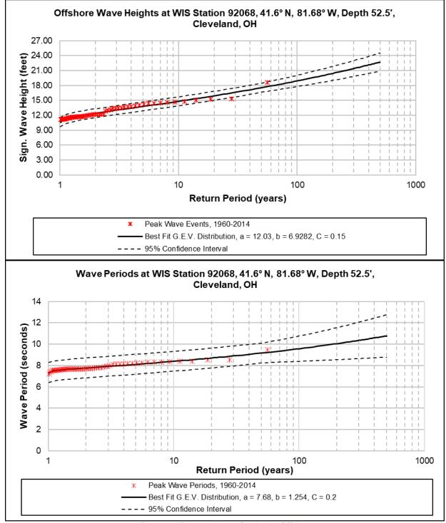
Figure 5: Extreme Wave Statistics Offshore
