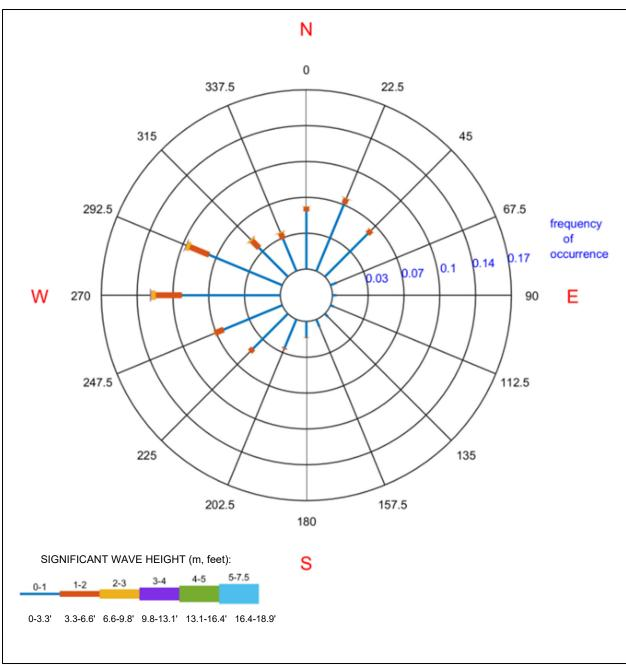
Figure 4: Wave Rose for WIS station 92068 (USACE)
