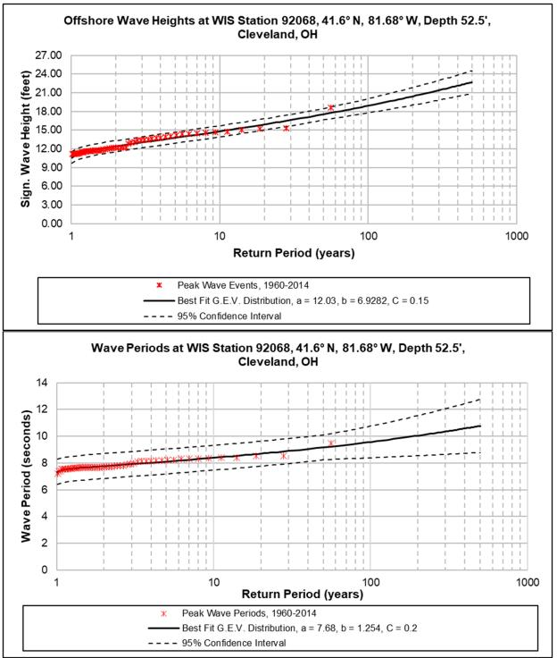
**Figure 5: Extreme Wave Statistics Offshore**
