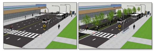
Figure 8. 'Before' and 'After' Views of a Midway Cycle Track Corridor
