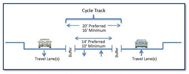
Figure 9. Midway Cycle Track Design Concept Cross Section
