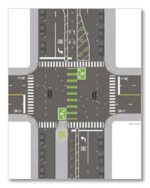
**Two-Stage Turn Box** Source: FHWA Separated Bike Lane Planning and Design Guide
