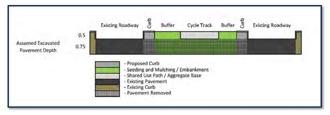
Figure 10. Midway Cycle Track Typical Section
