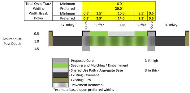
\*\*Using minimum widths will reduce Cycle track costs but increase resurfacing costs
