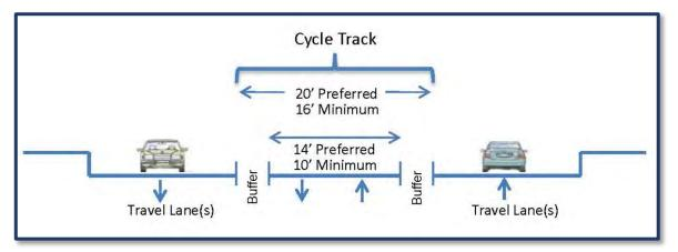
Figure 1. Midway Cycle Track Design Concept Cross Section
